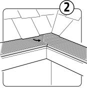
Repeat the process to install the other side of the miter, making sure the two sections meet flush at the front corner of the gutter. The mesh will overlap approximately 2 inches in the center.
