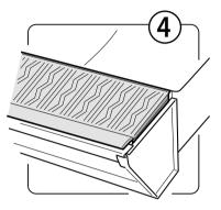
Make sure the entire gutter end is sealed to prevent debris and pests from getting under the gutter guards.
