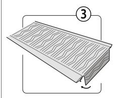
Bend and tuck the exposed mesh into the gutter. You can trim the mesh as needed to create a good covering.
