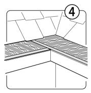
This is a completed inside corner. For heavy rain flow areas, you may need to use 14-mesh and/or add rain diverters.
