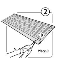
For piece B, trim back the aluminum rail about 1", leaving some mesh exposed.
