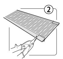
From the ground, trim back the aluminum rails where they are marked to expose the remaining mesh.
