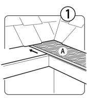
Slide piece A all the way into the inside corner of the gutter.
