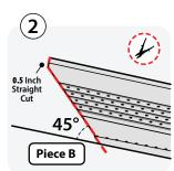
Cut the end of Piece B at 45 degrees. Next, notch the edge of the back wing in a 1/2 inch straight line. Place Piece B atop Piece A and check that the alignment has no gapping.
