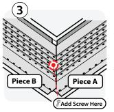
A completed outside corner should look like Image 3. For a tighter seal, place a screw through Piece B into Piece A to pull the pieces together.
