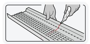
Use a new, or freshly sharpened pair of tin snips or a dremel to cut through the guard as needed. Not every piece of guard needs to be trimmed, only make cuts to end pieces to fit the length of the gutter. For safety, use protective gloves and make cuts while on the ground.
