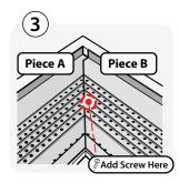
A completed inside corner should look like Image 3. Piece B should rest atop Piece A creating a seamless miter. For a tighter seal, place a screw through Piece B into Piece A to pull the pieces together.
