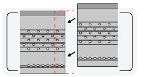
Slightly overlap the next guard so the perforated holes align with the previous piece. Follow the same screw pattern as the previous piece.
