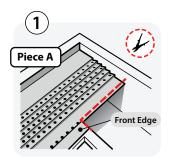
Trim the front edge of Piece A as shown in Image 1. Use the drain holes in the trough as a cut line. This will allow Piece B to fit properly atop Piece A.
