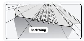
Drop the guard into the gutter with the front edge of the gutter guard resting on the front lip of the gutter. The guard is designed to rest on the gutter braces/brackets with a gradual upwards slope towards the house.
