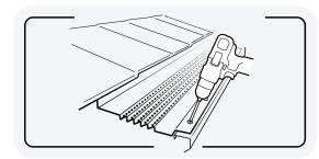
Using the provided 1/2 inch screws, secure the front edge of the guard to the gutter at both ends using the pre-drilled screw holes (3 inches from each end). Use 2 additional screws to fasten the front edge of the guard to the gutter.
